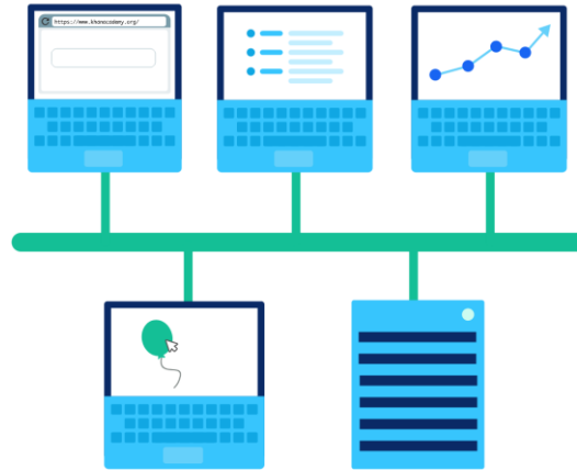
A LAN connected using a bus topology. The devices are connected with an Ethernet cable.
