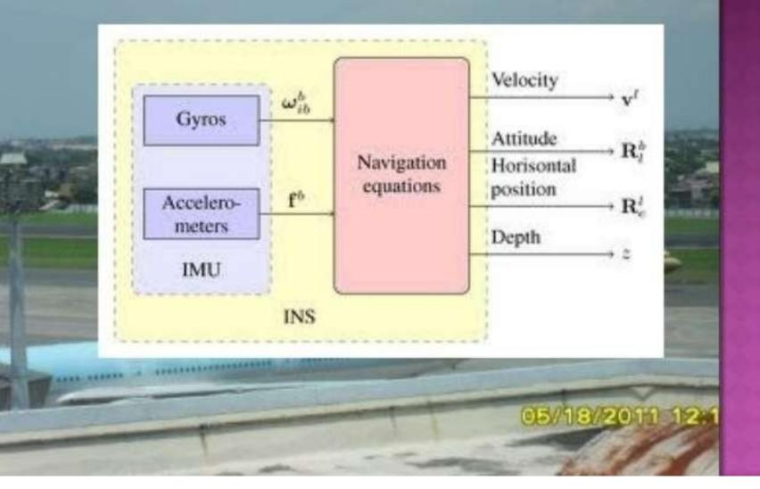
An inertial navigation system is a complex containing four basic components :-
