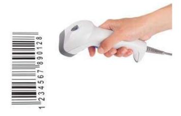
Bar Code Reader scans a bar code image, converts it into an alphanumeric value, which is then fed to the computer that the bar code reader is connected to.
