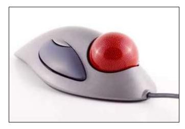
Since the whole device is not moved, a track ball requires less space than a mouse. A track ball comes in various shapes like a ball, a button, or a square.
