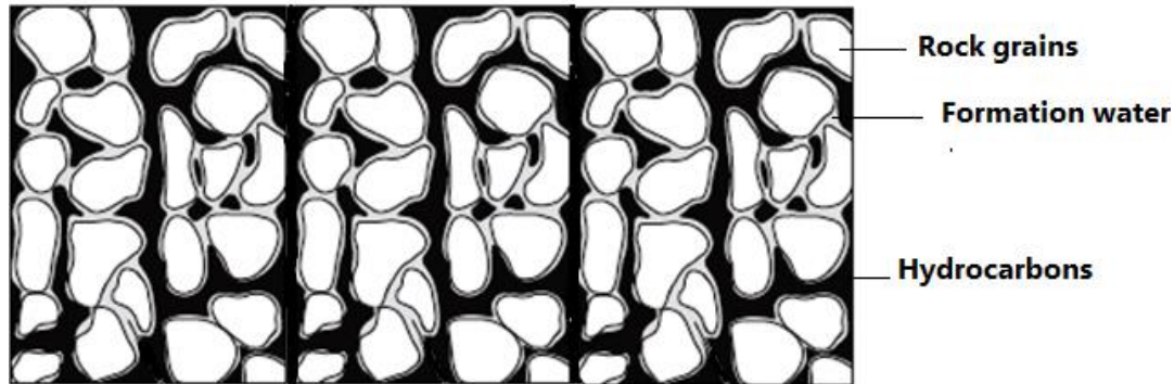
Section of a reservoir before drilling
