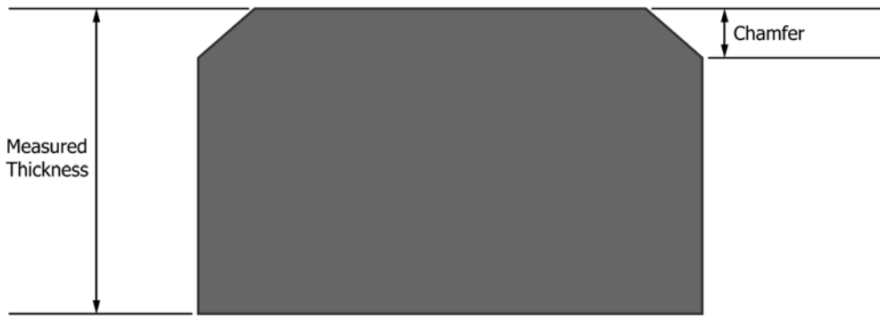
FIG. A4.1 Measuring Thickness of Paver with Chamfer (Section view from end of paver)
