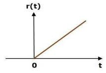
So, the unit ramp signal exists for all positive values of 't' including zero. And its value increases linearly with respect to 't' during this interval. The value of unit ramp signal is zero for all negative values of 't'.
