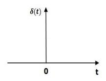
So, the unit impulse signal exists only at 't' is equal to zero. The area of this signal under small interval of time around 't' equal to zero is one. The value of unit impulse signal is zero for all other values of 't'.
