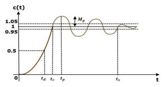
All the time domain specifications are represented in this figure. The response up to the settling time is known as transient response and the response after the settling time is known as steady state response.
