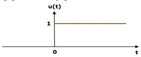
So, the unit step signal exists for all positive values of 't' including zero. And its value is one
