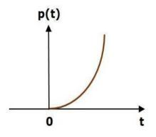
So, the unit parabolic signal exists for all the positive values of 't' including zero. And its value increases non-linearly with respect to 't' during this interval. The value of the unit parabolic signal is zero for all the negative values of 't'.
