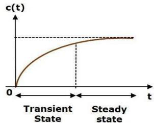
Here, both the transient and the steady states are indicated in the figure. The responses corresponding to these states are known as transient and steady state responses. Mathematically, we can write the time response c(t) as
