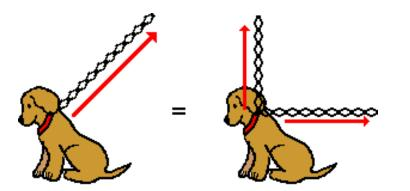
The upward and rightward force of the chain is equivalent to an upward force and a rightward force by two chains.
