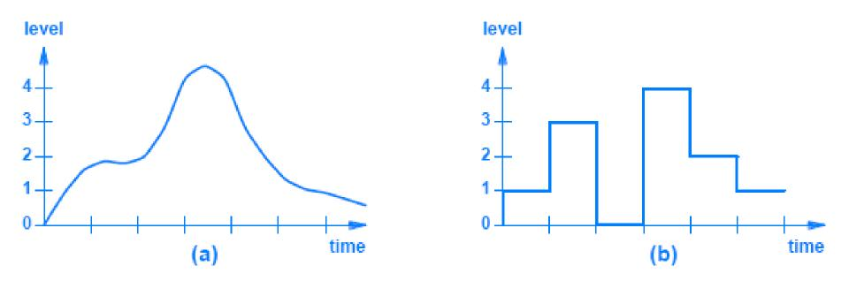
Figure 6.1 Illustration of (a) an analog signal, and (b) a digital signal.
