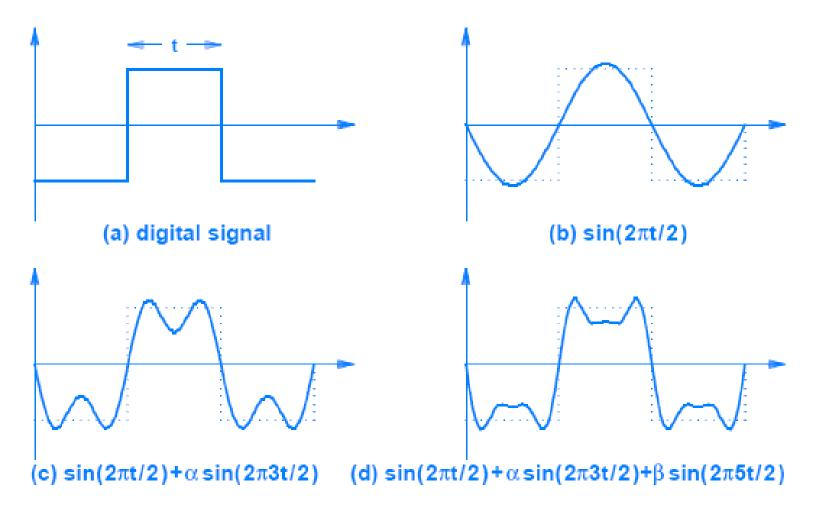
Figure 6.9 Approximation of a digital signal with sine waves.
