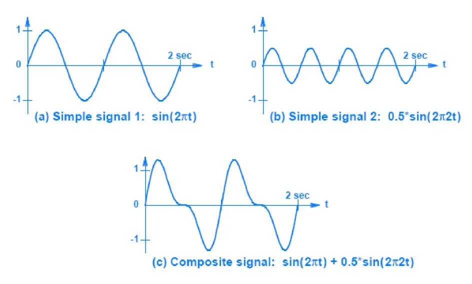
Figure 6.5 Illustration of a composite signal formed from two simple signals.
