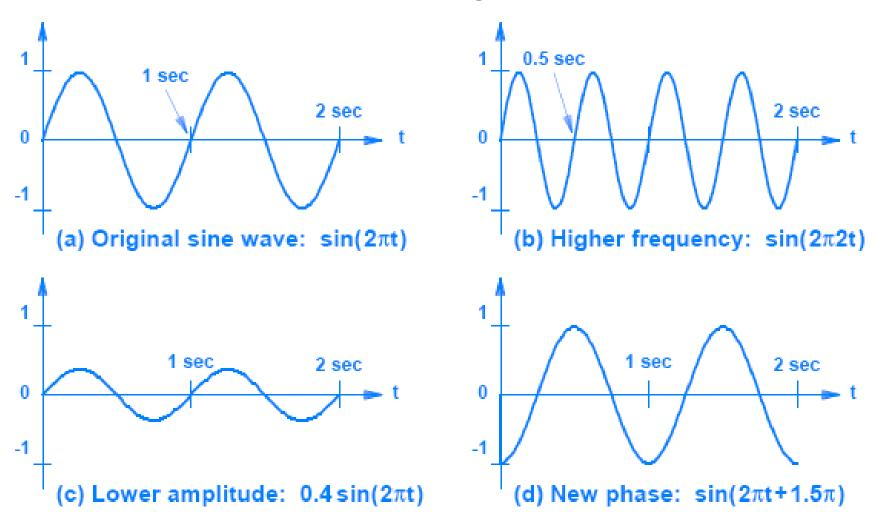
Figure 6.3 Illustration of frequency, amplitude, and phase characteristics.
