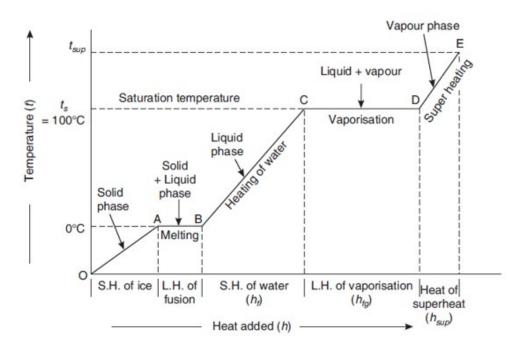
The temperature where equilibrium occurs at a given pressure level is called **saturated temperature**. The pressure where equilibrium occurs at a given temperature is called **saturated pressure**.
