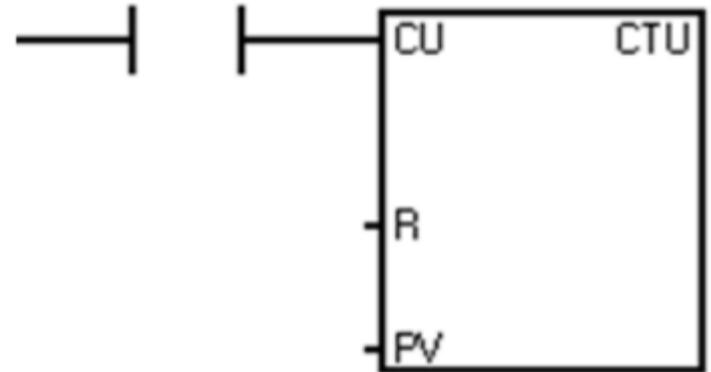
The counter will **not operate** on the trailing edge, or **on-to-off transition**, of the input condition
