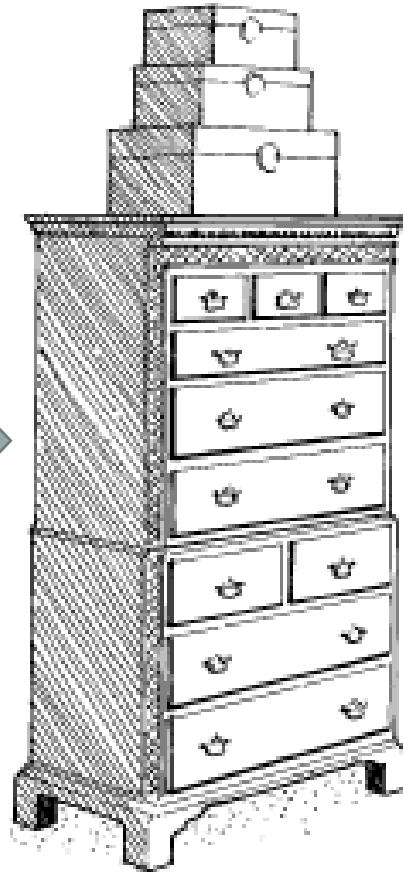
Figure 3.3 This chest is divided according to the golden section, just below the halfway mark.
