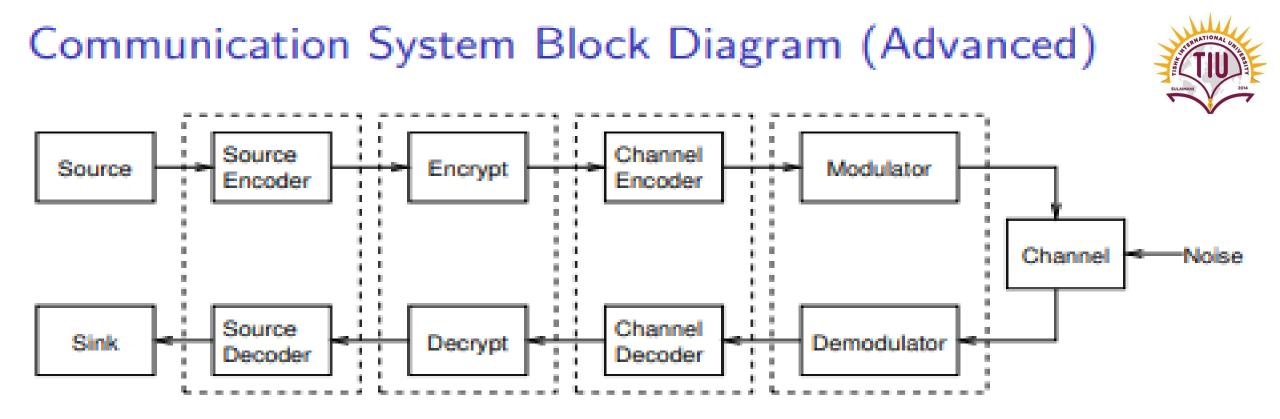
Source encoder compresses message to remove redundancy
