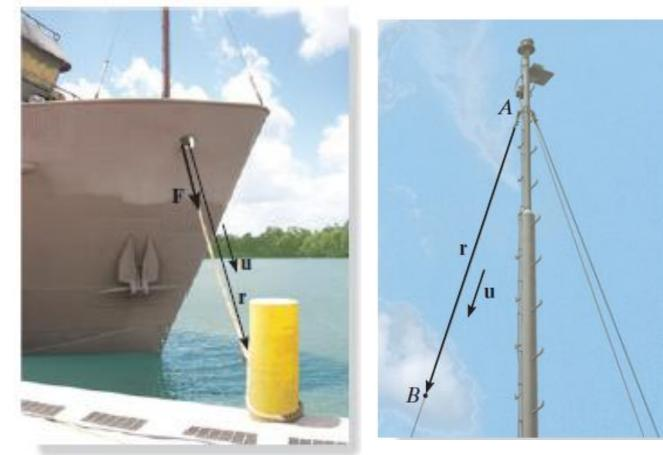
$$\mathbf{F} = F\mathbf{u} = F\frac{r_{AB}}{|r_{AB}|} = F\frac{(x_B - x_A)i + (y_B - y_A)j + (z_B - z_A)k}{\sqrt{(x_B - x_A)^2 + (y_B - y_A)^2 + (z_B - z_A)^2}}$$
