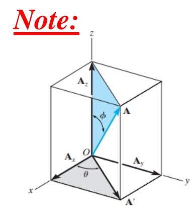
Sometimes, the direction of **A** can be specified using two angles,  $\theta$  and  $\phi$  (phi), such as shown in Fig. . The components of **A** can then be determined by applying trigonometry first to the blue right triangle, which yields
