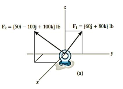
The coordinate direction angles  $\alpha, \beta, \gamma$  are determined from the components of the unit vector acting in the direction of  $\mathbf{F}_{R}$ .
