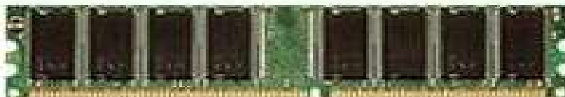
184 pin DDR DIMM
