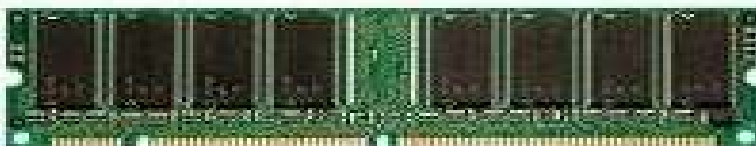
168 pin SDRAM DIMM
