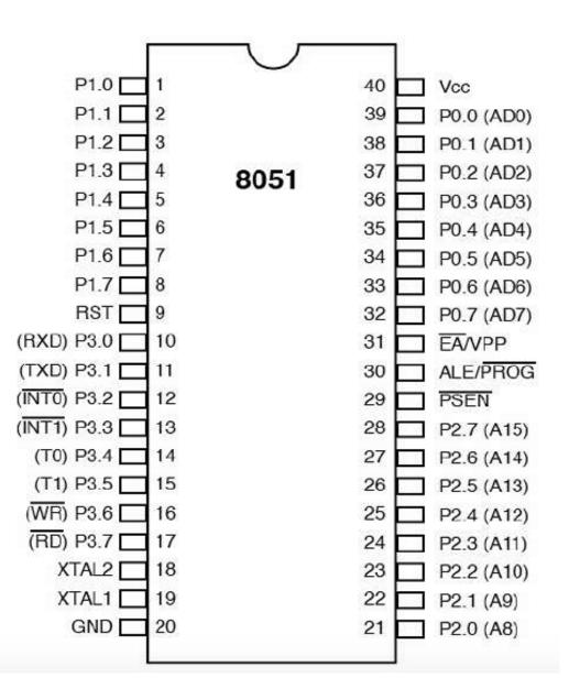
8051 microcontrollers have 4 I/O ports each of 8-bit, which can be configured as input or output. Hence, total 32 input/output pins allow the microcontroller to be connected with the peripheral devices.
