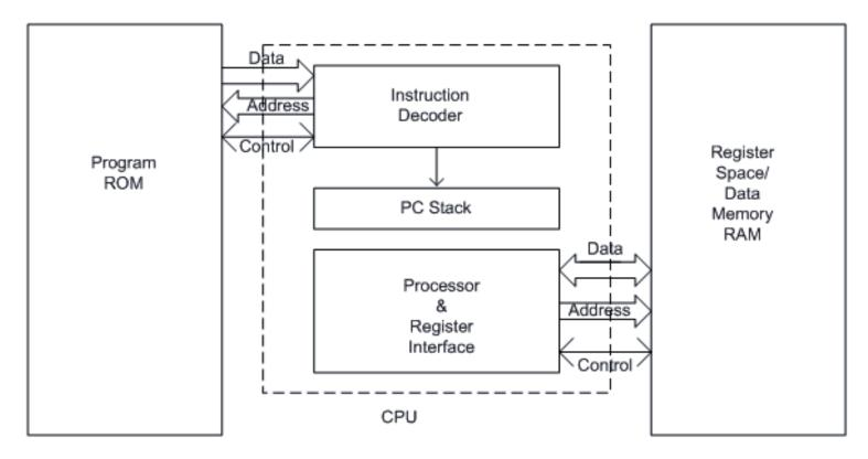
8051 microcontroller is designed by Intel in 1981. It is an 8-bit microcontroller. It is built with 40 pins DIP (dual inline package), 4kb of ROM storage and 128 bytes of RAM storage, 2 16-bit timers. It consists of four parallel 8-bit ports, which are programmable as well as addressable as per the requirement. An on-chip crystal oscillator is integrated in the microcontroller having crystal frequency of 12 MHz.
