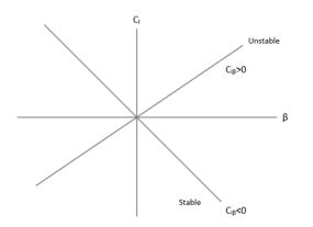
Explanation: Above diagram is illustrating the concept of roll stability. Typical lateral stability criteria can be observed in the diagram. Longitudinal stability is represented by using pitching moment curve. Lift curve will be used to provide relationship between lift and angle of attack. Drag polar will correlate drag and lift.
