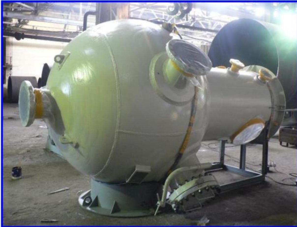
A typical spherical low-pressure separator
