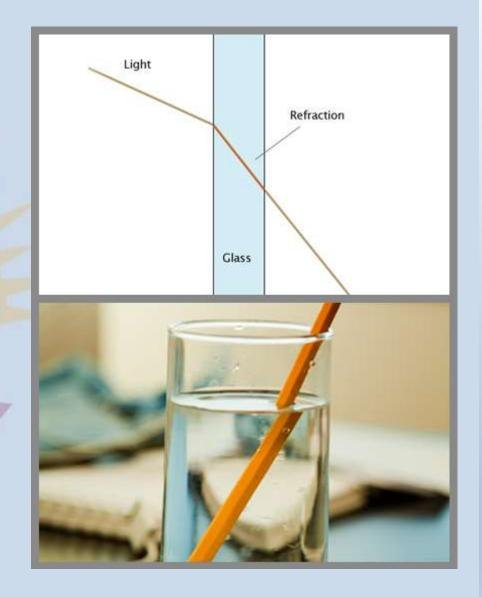
If a light beam meets a new material at an angle other than perpendicular. It bends, or refracted.
