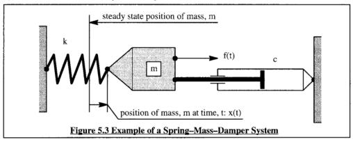
The equation of motion for the system of Figure 5.3 can be written as follows:
