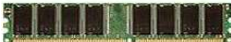
184 pin DDR DIMM
