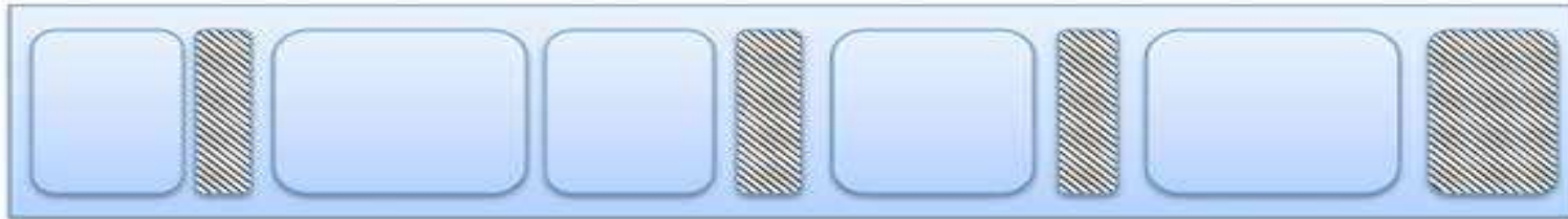
Fragmented memory before compaction
