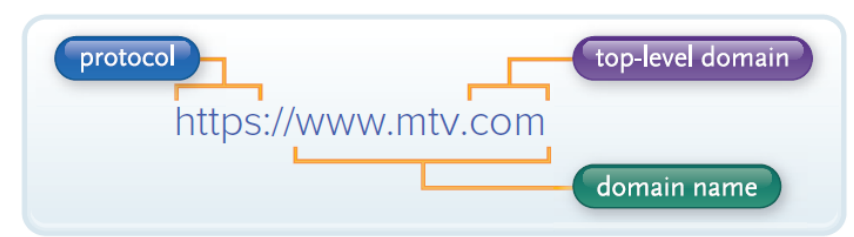
Figure 2-3 Basic parts of a URL
