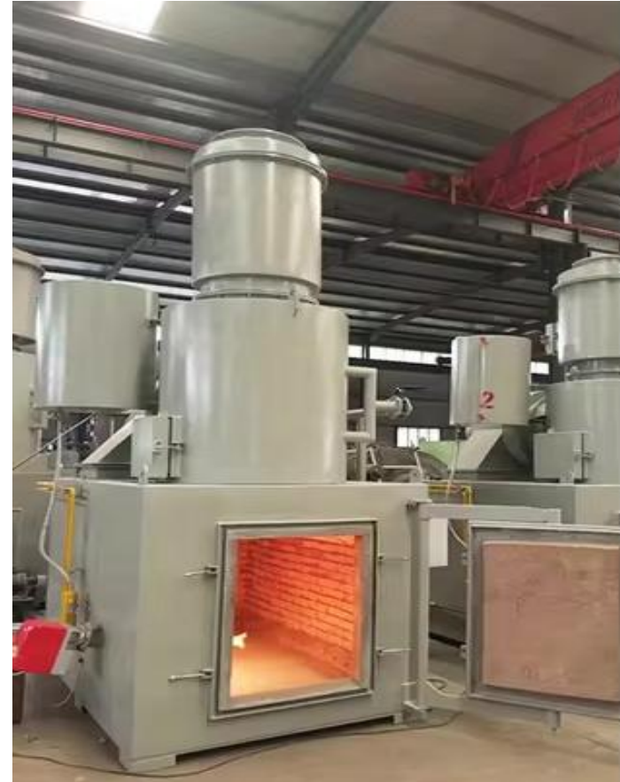
Medical waste incinerator
