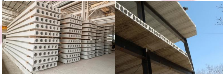
hollow-core precast concrete slabs
