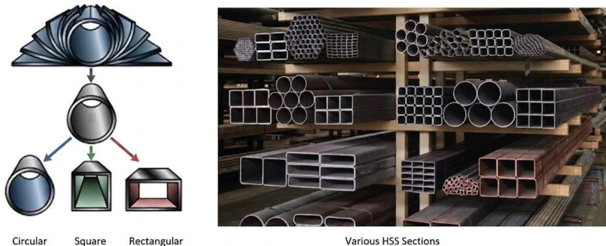
Common cold formed hollow structural sections (HSS)
